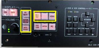
**ON**: When powering on a station, please allow one minute for the equipment to warm up. If the button is flashing, input cannot be changed.
